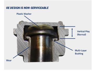
Premature slider (or telescoping) ball joint failures are a common occurrence on many late-model Dodge and RAM trucks and Jeep SUVs equipped with a straight or solid axle. The OE ball joints are not greaseable, which can increase the rate at which they wear. As the ball joint wears, looseness develops in the socket. Vertical movement of the stud is normal, but once radial movement (side-to-side or back-and-forth play) exceeds manufacturer specifications, it's time to replace the ball joint.
